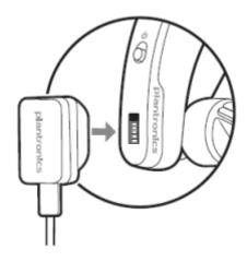
2. Attach cable to the USB wall charger or laptop for 90 minutes. Once fully charged, the LEDs will turn off.
