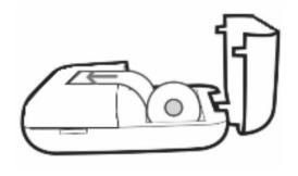
2. Cover the paper bin, the machine can automatically absorb paper after normal use.
