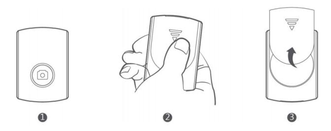
You can take over 30.000 photos with the battery that comes with the selfie stick. If you leave the remote unused, it will enter the sleep mode after 3 minutes and power off after 6 hours. This increases the life of the remote's battery.
