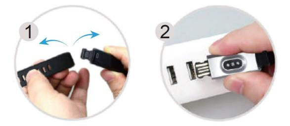
Insert the charging plug of the tracker into the USB port for charging. Make sure the pins on the charging plug contact those in the USB port.
