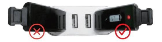
If the activity tracker is on low battery, connect it to an adapter for charging. The tracker will automatically boot up once fully charged. USB charger requirements are:
