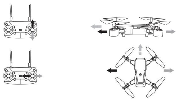
The right analog controls moving the drone forward and backward and also flying to the right and to the left.
