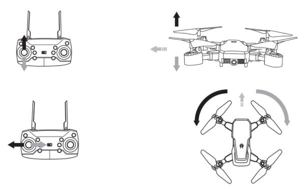
The left analog controls the rising and falling of the drone and also turning the drone left and right.
