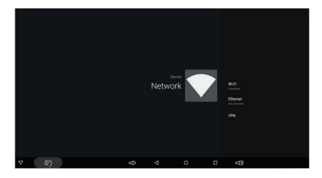
To set up the Ethernet connection, go to Settings -> Network and select Ethernet to open the LAN settings. Then plug the LAN cable and it will automatically connect to the network.
